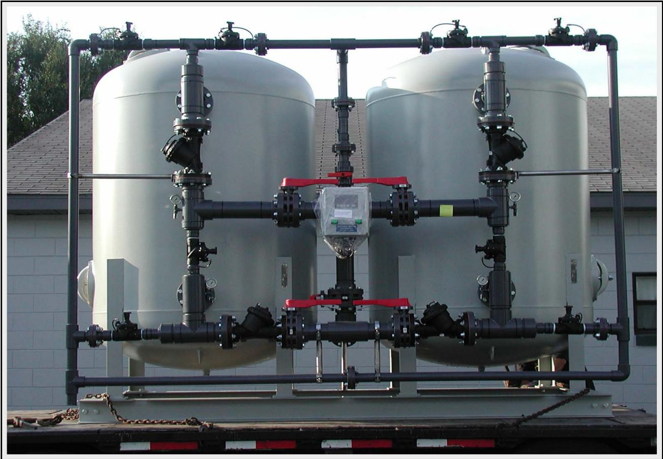
The ASDC-6060-4/2/PVC is one of our largest water softeners. The ASDC-6060-4/2/PVC features 2" regeneration and 4" outlet Schedule 80 PVC face piping, a twin alternating stager and controller which can be controlled with air or water pressure, a flow sensor, and optional flow transmitter capability. This softener also features Carbon Steel Epoxy lined ASME code tanks, PVC Diaphragm valves, and Viton/EPPM seal construction.
